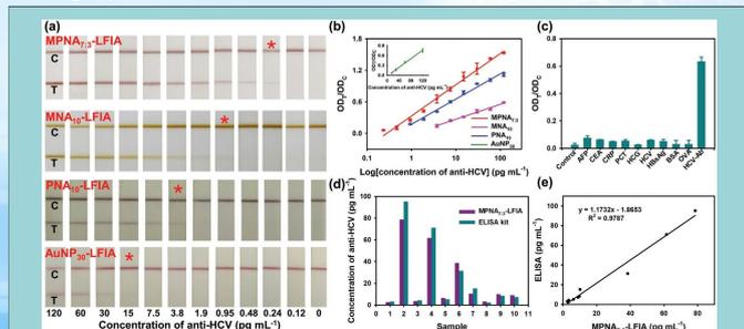
Figure 3. The detection performance of all four LFIA strips, including MPNA<sub>7.3</sub>-LFIA, MNA<sub>10</sub>-LFIA, PNA<sub>10</sub>-LFIA, and AuNP<sub>30</sub>-LFIA in the detection of anti-HCV.
