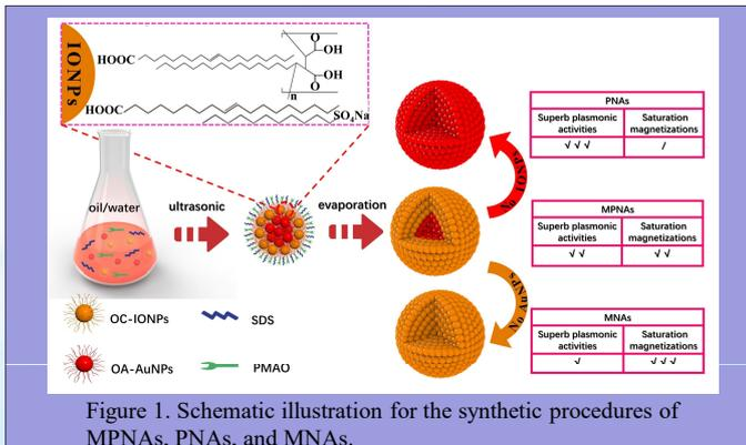
Figure 1. Schematic illustration for the synthetic procedures of MPNAs, PNAs, and MNAs.
