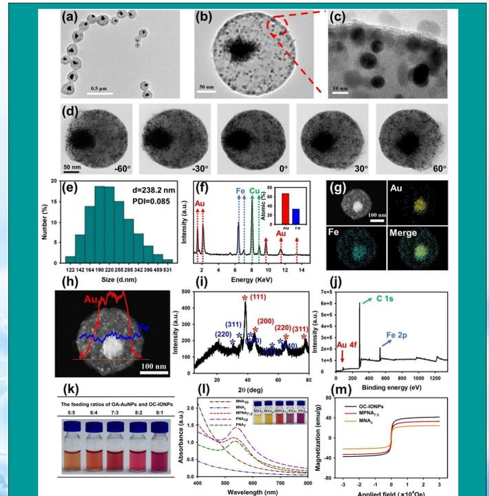
Figure 2. Characterizations of the MPNAs. (a-c) TEM images; (d) Tomographic TEM images; (e) Hydrodynamic Diameter; (f) EDS spectroscopy; (g) HAADF-STEM EDS elemental mapping; (h) EDS elemental line scan; (i) Power XRD pattern; (j) XPS analysis; (k) feeding ratios of OA-AuNPs and OC-IONPs; (l) plasmonic activities; (m) magnetic activities.
